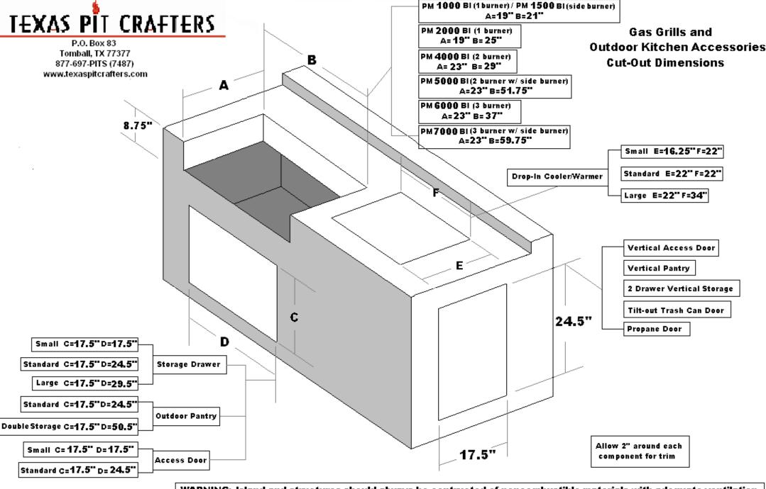
WARNING: Island and structures should always be contructed of noncombustible materials with adequate ventilation.
