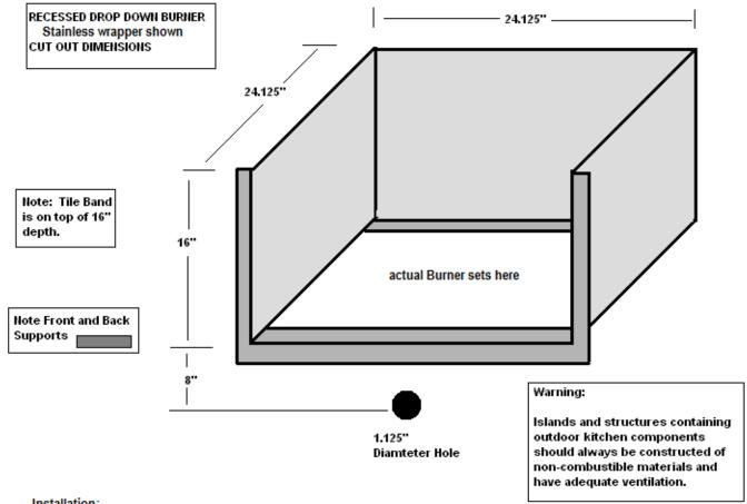
Installation: The front edge of Recessed Burner slides back into opening
